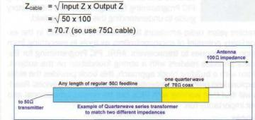
**FACT 6.** Parallel coaxes can be utilised to match a number of situations with a little creativity when the formula comes out to non-standard transmission line. This diagram shows how to make up a  $35\Omega$  quarter wave matching section, required to match the  $25\Omega$  of two paralleled  $50\Omega$  antennas to a  $50\Omega$  feedline.
